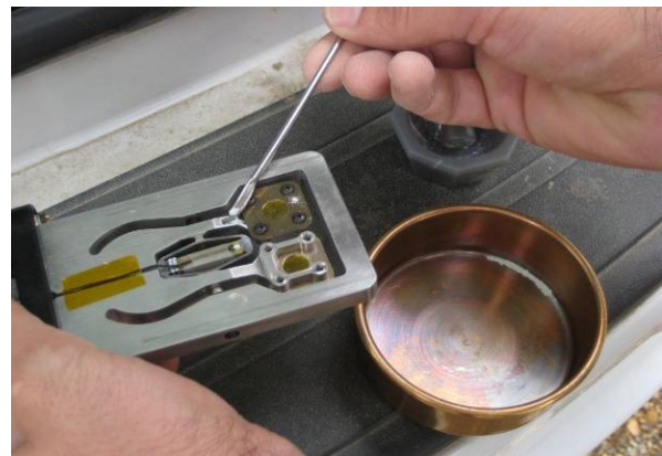
Figure 2: Loading sample into the piezoelectric-actuated cell.
