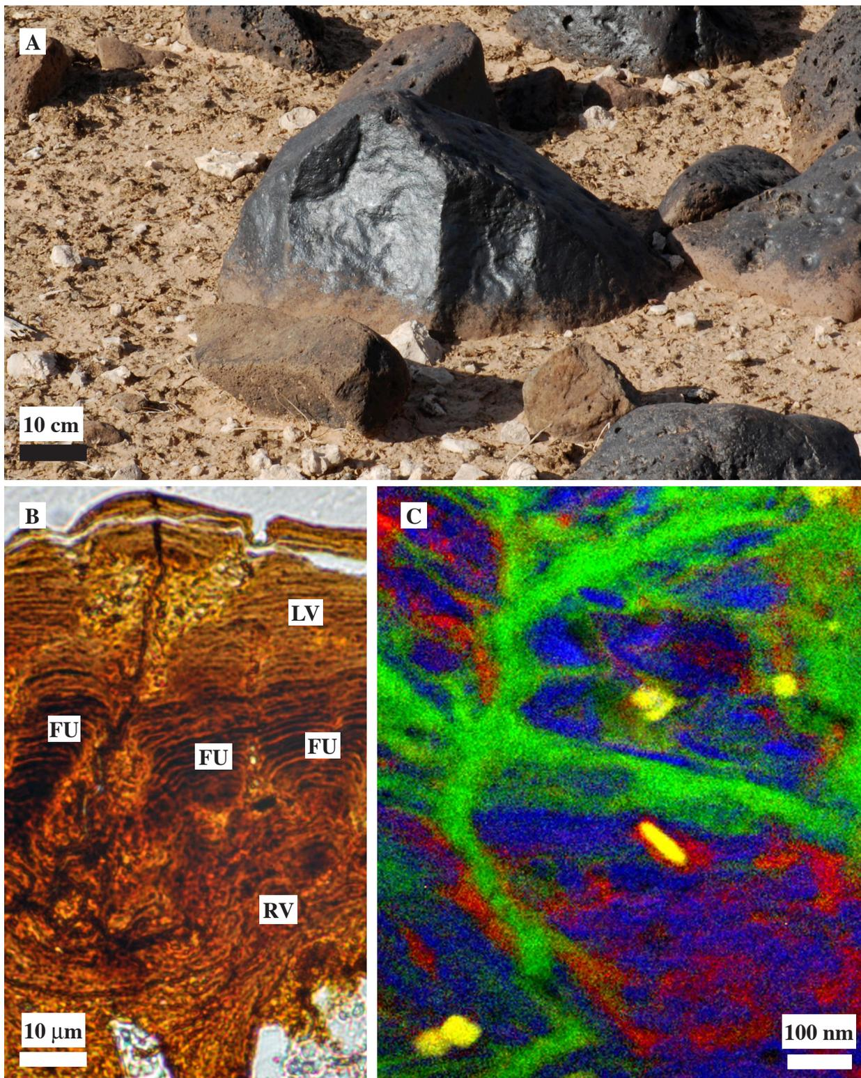
A) Photograph of a varnish-covered boulder from southern Arizona. B) Ultrathin section of desert varnish showing the layered flaring-upward structures (FU), layered varnish (LV) parallel to the air-varnish surface (LV), and rubbly bottom between varnish and underlying rock (RV). C) Energy-filtered TEM image from a thin section of desert varnish prepared using a focused ion-beam and showing the distribution of Fe (red), Mn (green), Si (blue), and Ti (yellow).
