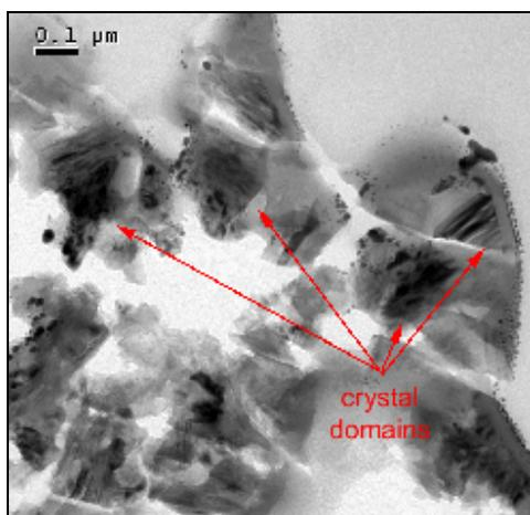
**Figure 3.** BF image of an area of a KJG SiC X grain. Multiple crystal domains (arrows) are visible within the grain. Intensity variations between domains are due to orientation-dependent diffraction contrast.
