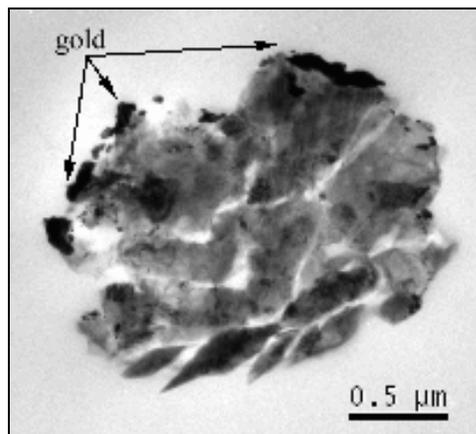
**Figure 2.** Bright field (BF) TEM image of an ultramicrotome slice of a KJG SiC X grain. Because SiC is so hard, the grain shatters when sliced, but individual crystal domains are visible within the fragments. The black areas at the top of the slice are Au deposits from NanoSIMS analysis.
