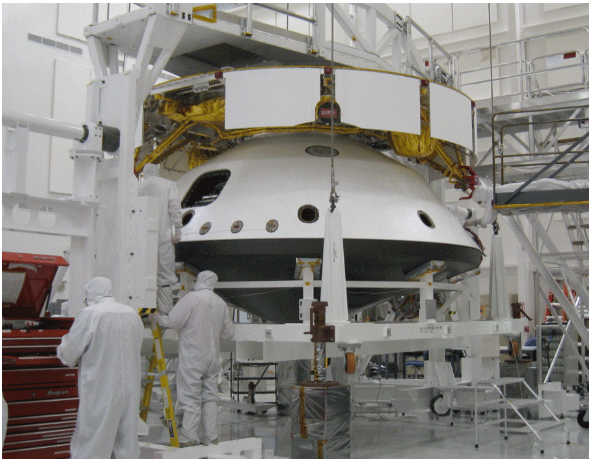
Figure 1. The Mars Science Laboratory cruise stage (top), aeroshell (middle), and heat shield (bottom, not flight model) in assembly and testing at JPL. Inside the aeroshell are the completed descent stage ("sky crane") and rover body.
