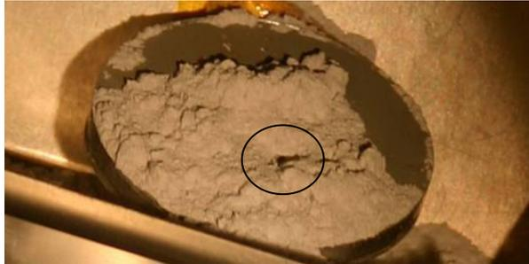
Fig. 2. Basalt target (30 mm dia) loaded with dust, shown after analysis in a simulated Mars atmosphere. LIBS analysis spot is circled.
