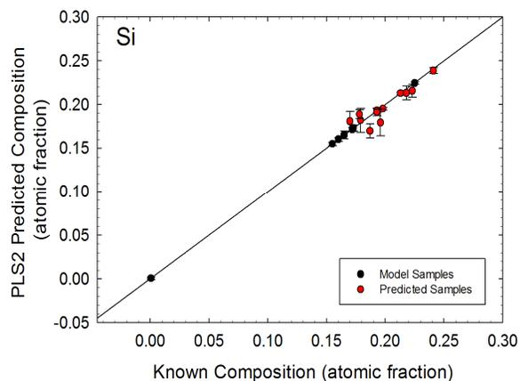
Fig. 3. Silicon calibration curve of a subset of the standards run, using partial least squares (PLS) analysis.
