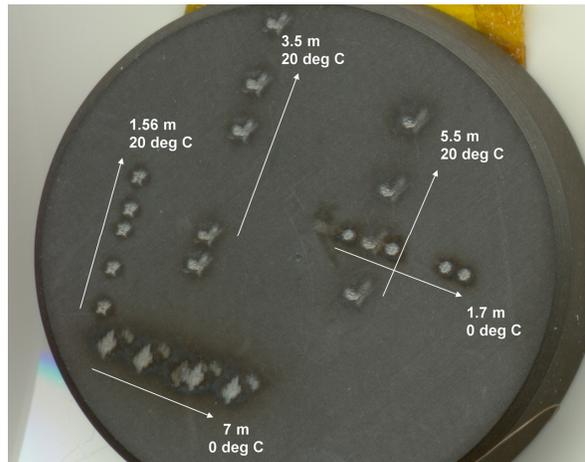
Fig. 1. Rows of laser pits (50 shots each pit) in 22 mm diameter graphite standard placed at various distances from the instrument.
