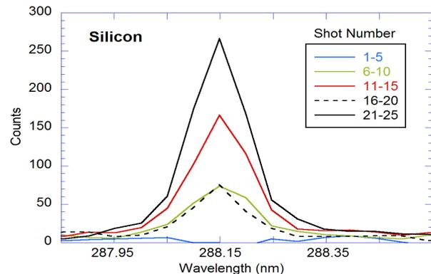
Fig. 4. In-growth with successive laser shots of the Si emission line from the basalt sample covered with 2-3 mm of dolomite dust at 3.5 m distance.
