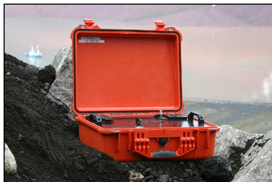
Figure 2. inXitu's Terra portable powder XRD instrument deployed in Spitsbergen during the AMASE 2007 expedition.
