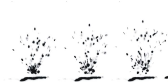
Fig. 1 Snap shots of a dust eruption from a basalt dust bed (lower line) illuminated by a halogen lamp with several kW/m 2 (colour inverted, illuminated dust particles appear black). The lowest big dust aggregate disintegrates further while airborne. Scale is about 2cm x 2cm.
