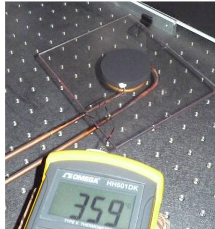
**Figure 4 Evaluation of a new calibration target with the induction heating system**
