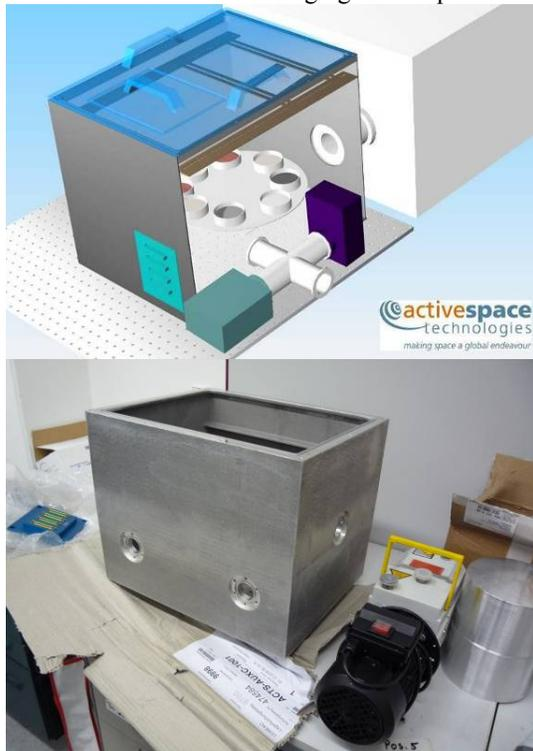
**Figure 3 Top: Schematic view of the new planetary simulation chamber- Bottom: Chamber casing at manufacturer**
