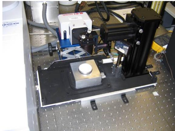
**Figure 2: Open emissivity chamber (top cover removed)**
