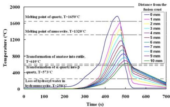
Figure 2: Analytical model of the temperature evolution through the sample thickness. The transition temperatures of the minerals have been reported.
