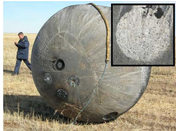
Figure 1: The STONE 6 artificial meteorites after landing in Kazakhstan. The samples are embedded at the apex of the heat shield, around the ablation point. A micrograph of the sedimentary rocks sample after landing is shown in insert.
