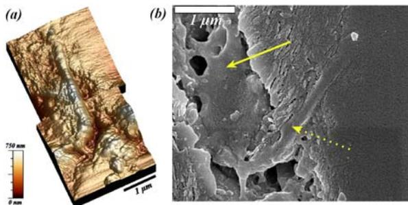
Figure 3: (a) AFM image of a filamentous microfossil and (b) the corresponding SEM image showing the EPS (solid arrow) surrounding the structure (dash arrow).
