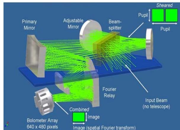
**Figure 1.** The ATMS Warm Detector Array Breadboard optical layout. The instrument dimensions are approximately  $160 \times 220 \times 370 \text{ mm}^3$ .
