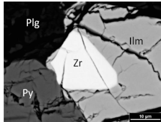
**Fig.1** BSE image of a zircon (Mil-Z12) with typical 120° intergrain boundaries for the mineral paragenesis with ilmenite (ilm), pyroxene (py), and plagioclase (plg).
