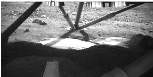
Figure 1 “Holy Cow” as imaged by the RAC. Thruster rockets can be seen at the upper edge of the image.
