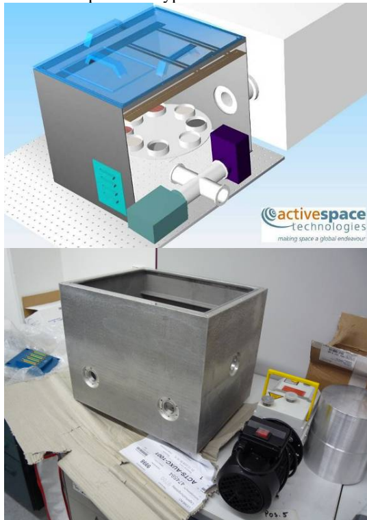
Figure 2 Top: Schematic view of the new planetary simulation chamber- Bottom: Chamber casing at manufacturer
