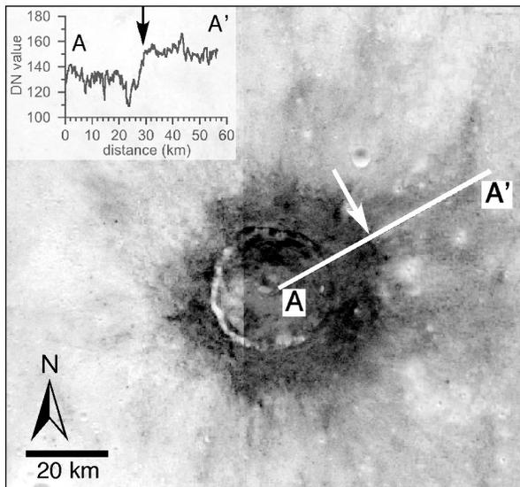
**Figure 1.** Iron concentration map of Timocharis Crater (33 km in diameter) derived from Clementine UV-VIS data [12]. Radial profile A-A' shows distinct step (arrow) from low iron ejecta inferred to represent the transition from sub-mare basement material to more iron-rich basaltic ejecta.
