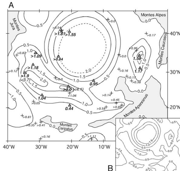
**Figure 2.** (a) Basalt isopach map of Mare Imbrium. Filled triangles represent craters examined in this study, crosses represent locations of partially flooded craters examined previously [6]. All data labels are given in km; contour interval is 0.5 km. The position of the 2.0 km contour is not well constrained and is depicted with a dashed line to reflect this uncertainty. (b) Simplified basalt isopach map of Mare Imbrium determined from partially flooded craters (after [6]).
