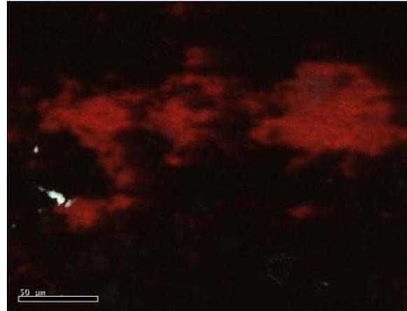
**Figure 6: Red CL activity in calcite. The pale white features at lower left may be artifacts, perhaps due to surface charging or a defect in the carbon coating of the section.**
