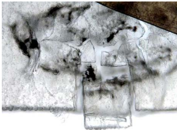
Fig.1: Sample C2092,3,0,0 dissected from track 80 (lower part of the micrograph). This track have a large bulbous shape (about 5 mm length and 2 mm wide).
