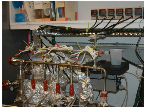
**Figure 1:** Manifold where Genesis samples were baked for 322 days. Each finger contained 2 pieces of polished Al and 1 piece of AloS.
