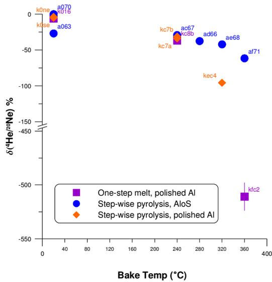
**Figure 2:** Bulk (total of all step-wise pyrolysis steps) ratios ( $^3\text{He}/^4\text{He}$  and  $^4\text{He}/^{20}\text{Ne}$ ) normalized to reference unbaked AloS sample (a70). Labels denote individual samples. X-axis refers to the baking temperature the sample was held at for the 322-day diffusion experiment, not the step-wise pyrolysis temperature. Error bars are  $1\sigma$  statistical uncertainties.
