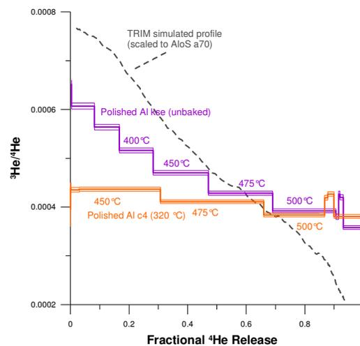
**Figure 4:** Helium release profiles for AloS (top) and polished Al (bottom) compared to the simulated depth profile given by TRIM code [5]. Each horizontal bar represents the measured ratio of a pyrolysis step, with the temperature of some of the larger steps labeled on the plot. Error bars are  $1\sigma$  statistical uncertainties.
