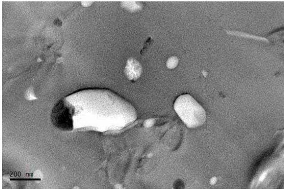
**Figure 2.** Low magnification TEM image of voids in matrix olivine from NWA1628. Many of the voids are associated with sulfide crystals. Dislocations are present locally in the olivine.
