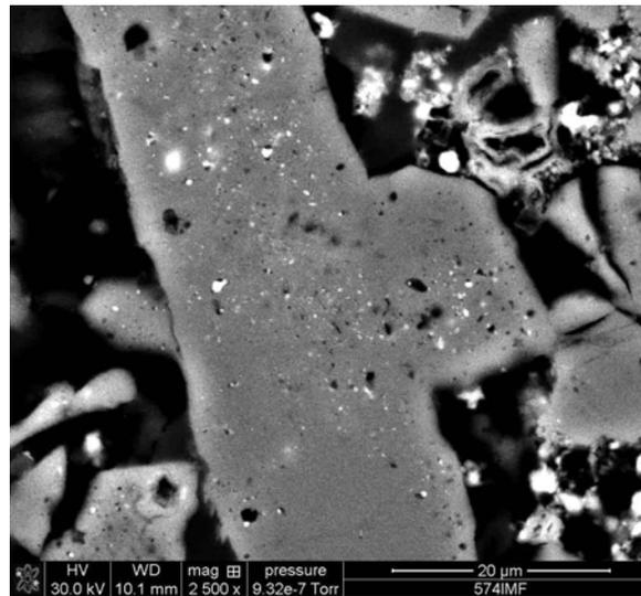
**Figure 1.** FESEM image of elongate olivine grain in the matrix of NWA 1628, showing heterogeneous distribution of inclusions. The dark inclusions appear to be vesicles and the high Z inclusions are dominantly FeNi sulfides.
