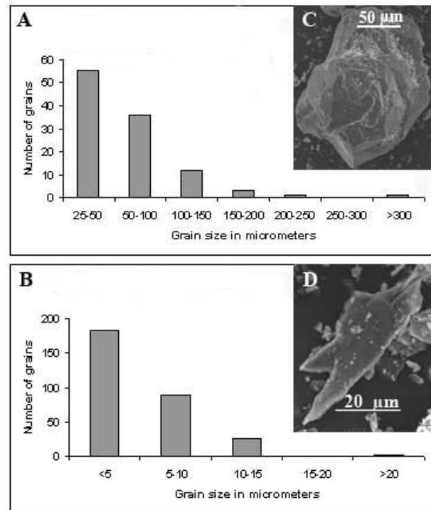
Figure 1: Grain size distribution of breccia matrix. A) Grain size distribution on 500 μm scale; B) Grain size distribution on 20 μm scale; C) SEM image of dominating sub-rounded quartz crystal; D) SEM image of irregular silica shard.
