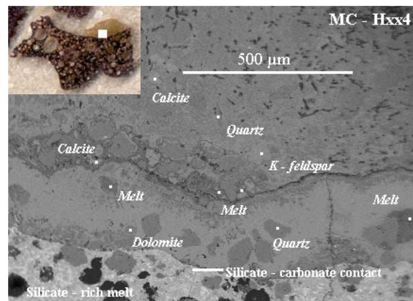
Figure 2. Backscattered electron image of the carbonate-rich coating (bulk of image) on a silicate melt particle (bright unit along bottom of image) on particle MC-Hxx4. The inset shows a plane-light view of the entire particle.
