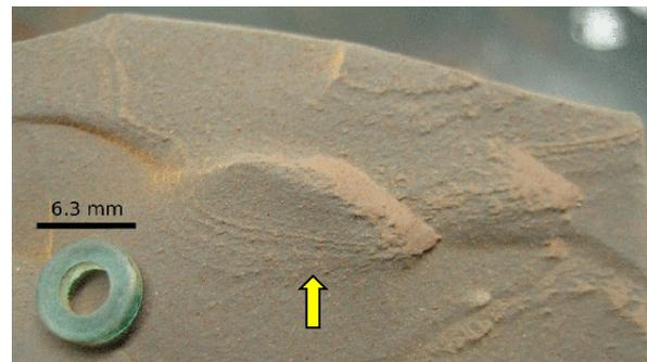
**Figure 2:** Enhanced lamina contrast on a mudstone after seven weeks inside abrasion chamber with lava rock as eroding medium.
