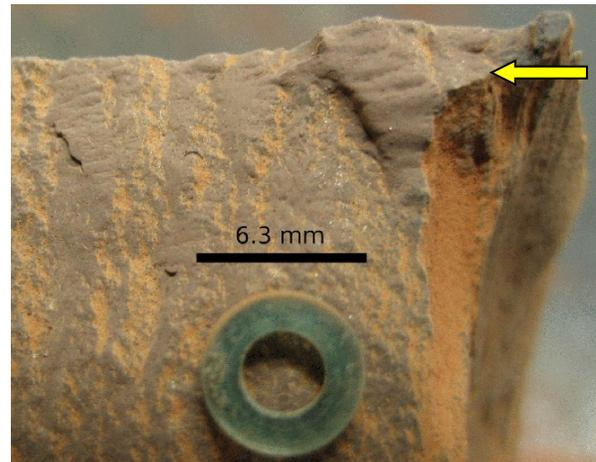
**Figure 1:** Mudstone exhibiting polished surfaces after seven weeks inside abrasion chamber with lava rock as eroding medium.
