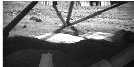
*Fig. 1 - A robotic arm camera image under the lander showing several areas of ice-rich material exposed by the descent thrusters. The exposed icy surface was named "Holy Cow." The view is to the south.*
