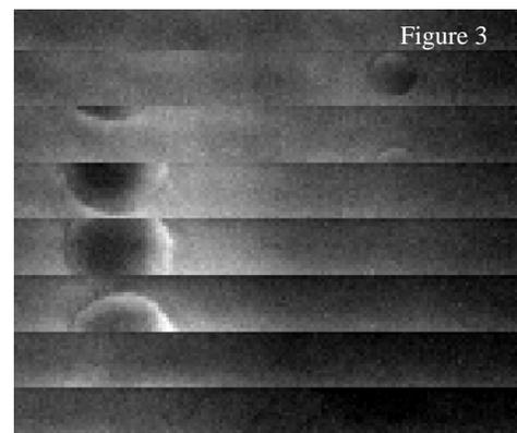
Neither frame nor pushbroom cameras exhibit the visualization difficulties of raw products like pushframe cameras. Special software must be written to break apart and reorganize the framelets just for simple viewing. Commercial-off-the-shelf (COTS) and open source software typically lack support for this esoteric file structure. Therefore, basic image selection and analysis becomes a much more difficult task when compared against traditional cameras.
