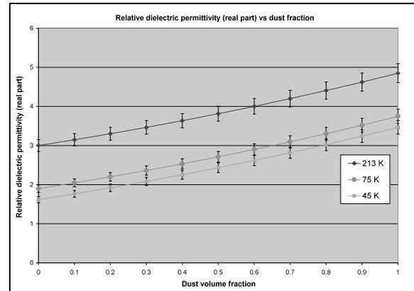
Figure 1: Relative dielectric permittivity as a function of dust fraction (real part).
