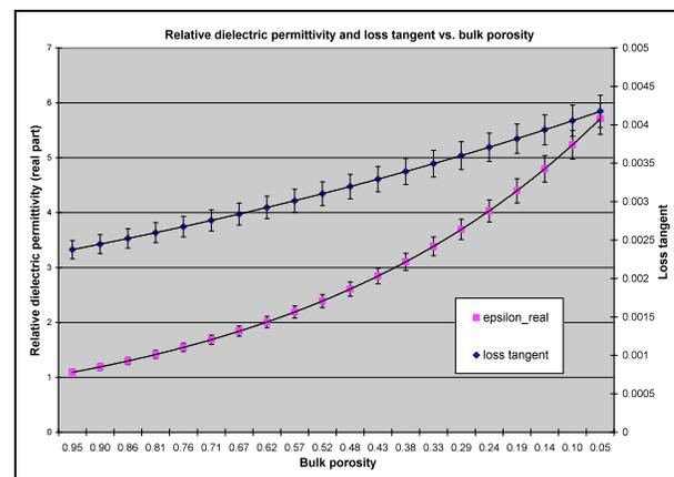
Figure 2: Relative dielectric permittivity as function of bulk porosity
