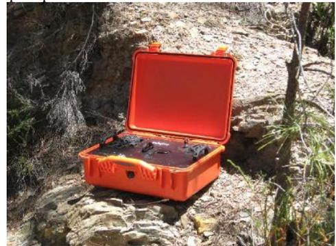
**Figure 2.** Terra portable XRD/XRF instrument deployed at the same location.
