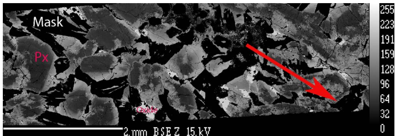
Fig 1. Backscattered electron image of NWA 5298 Arrow shows preferred orientation of pyroxene grains. Px = pyroxene, Mask = maskelynite, oxide = Fe-Ti oxide.
