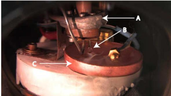
**Figure 2:** The methane reservoir (top panel labeled A in the bottom picture) is in the Titan environmental chamber. The drop comes out of the capillary (B) and falls on the copper stage (4" diameter) or onto ice substrate (C).
