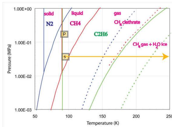
**Figure 1:** Stability domain of nitrogen (blue), methane (red) and ethane (green) in a  $(P,T)$  plane. The dashed lines show the stability of the different clathrates. The orange rectangles show the conditions in the reservoir ( $p$ ) and on the stage ( $s$ ). The arrow shows the evolution when the stage heats up at the end of each experiment.
