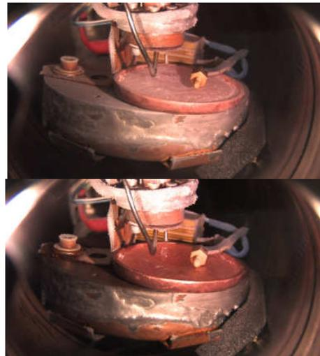
**Figure 3:** When water ice (top picture) is wetted by liquid methane, the methane is absorbed in the ice and causes change in its optical properties (bottom picture).
