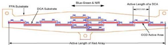
**Fig. 1.** HiRISE CCD structure on its focal plane. (Alfred McEwen 2007).
