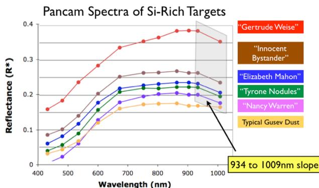
**Fig. 1.** Example spectra of materials confirmed as Si-rich by Mini-TES and/or APXS (plus typical Gusev dust for comparison).
