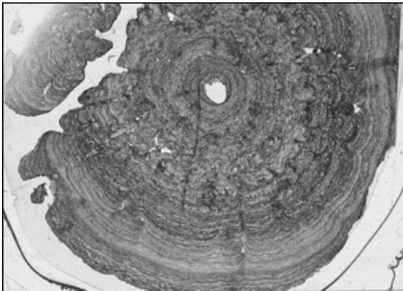
**Figure 1. Sample 028 in plane-polarized light, showing alternation between smooth and rough laminae. Width of field of view 3.5 cm.**
