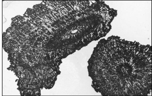
**Figure 2. Sample 009 in plane-polarized light showing radially distributed elongate carbonate crystals with void space and dark clay material. Width of field of view 3.5 cm.**
