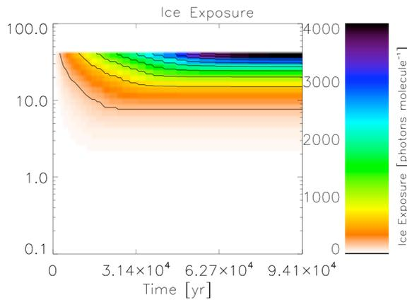
**Figure 1:** Exposure of ices in the proto-solar disk. Simulation runs for  $10^5$  years at a UV flux of  $10^6 G_0$ . A standard Hayashi profile and disk of mass  $0.015 M_{\text{sol}}$  is assumed. By the simulation end, ices in the outer solar system ( $>30$  AU) have received a mean dose of  $\sim 4000$  photons/molecule ( $5 \times 10^5$  eV/molecule). The contours flatten by the simulation end because rapid grain growth locks up exposed surface area into larger bodies.
