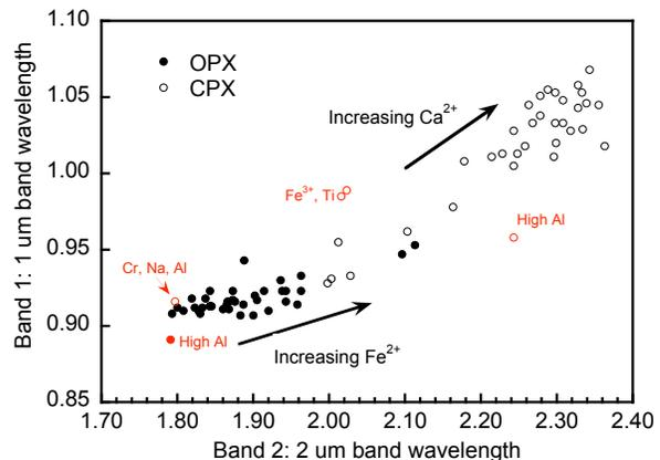
**Fig. 2.** Band 1 and 2 centers for a suite of natural pyroxenes, measured and analyzed by Adams [1974] and Cloutis and Gaffey [1991].
