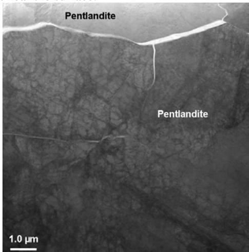
Figure 3. Bright-field STEM image of part of the FIB section from ROI-B. The pentlandite near the surface (top) shows uniform contrast, whereas that on the bottom is heterogeneous and reveals the detailed structure.
