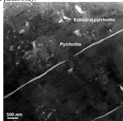
Figure 4. Bright-field STEM image of part of the FIB section from ROI-C. Euhedral pyrrhotite grains occur parallel to one another.
