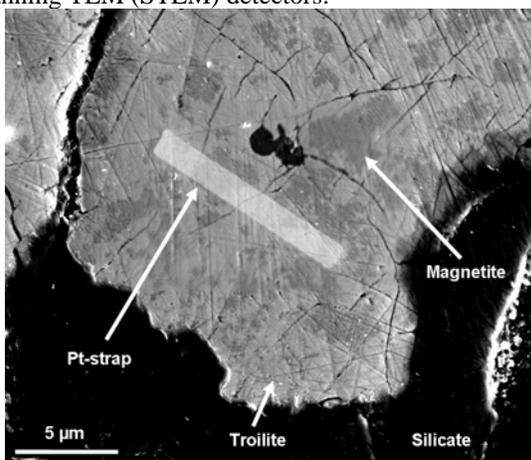
Figure 1. BSE image showing Pt-strap superimposed over a sulfide assemblage in Ch11, ROI-A. EMPA suggests dark patches are likely magnetite, while lighter areas are troilite.
