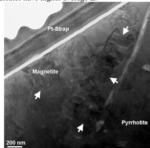
Figure 2. Bright-field TEM image of part of the FIB section from ROI-A. Magnetite occurs surrounded by pyrrhotite. The boundary of the magnetite assemblage is marked by white arrows.
