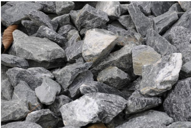
Below: Close up of same box showing the various shapes possible in a single-sized deposit.
