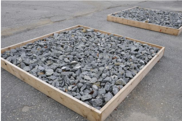
Above: Rock box containing natural samples of granite sieved to 6 inch minus size.
