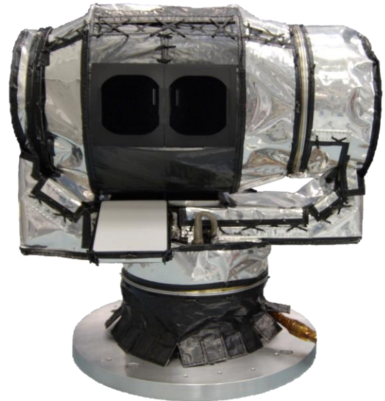
Figure 1: Diviner Lunar Radiometer. Diviner's optics are contained in the central drum behind the apertures. The azimuth and elevation actuators can each rotate 270°. The white surface is the solar calibration target, which is used for photometric calibrations. Blackbody calibration targets, used for radiometric calibrations, are located in the yoke.
