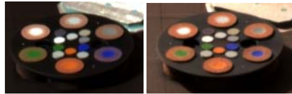
Fig. 2: iSweep no. 2 on Phoenix sol 13 and 60. Dust is settling primarily on the ring of the color chips as expected, leaving the center very clean.
