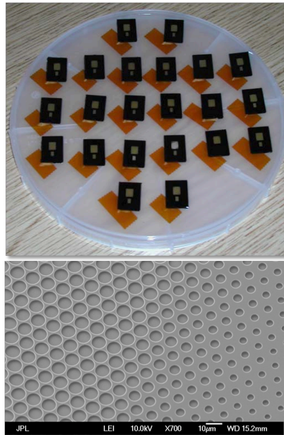
Figure 3. Top: Photo of test die to investigate membrane burst pressures for a series of different membrane designs. For a given die, the small membrane transmits X-rays to the sample and the larger membrane transmits photoelectrons to the analyzer. Bottom: SEM shows ultra-thin nitride window array for electron transmission.
