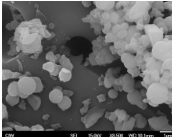
**Figure 3:** SEM image of Formose polymer hydrothermally processed to 250 °C highlighting the presence of abundant micron and sub-micron organic spheres.
