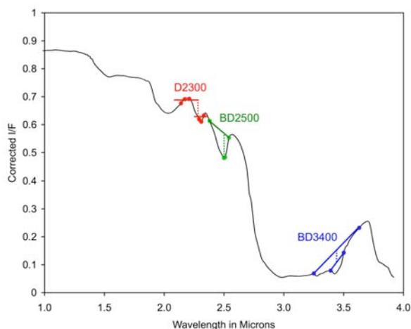
Fig. 1. Example of our approach used to compute carbonate spectral parameters using a laboratory spectrum of magnesite + hydromagnesite. Here the 2.5- $\mu\text{m}$  and 3.4- $\mu\text{m}$  band depths and the falloff of reflectance into the 2.3- $\mu\text{m}$  band in this spectrum are determined.
