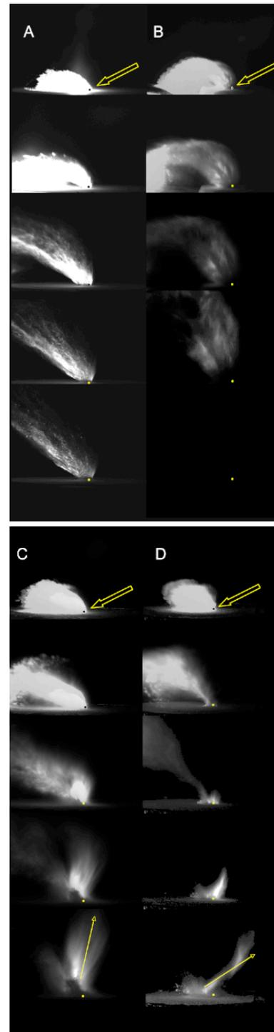
**Figure 1:** Evolution of the early stages of formation (40, 72, 142, 253, and  $400 \mu\text{s}$  after impact) for impacts into dry sand (A), dry ice (B), perlite/dolomite mixture (C), and target B covered by a layer of dry perlite dust (two projectiles thick).
