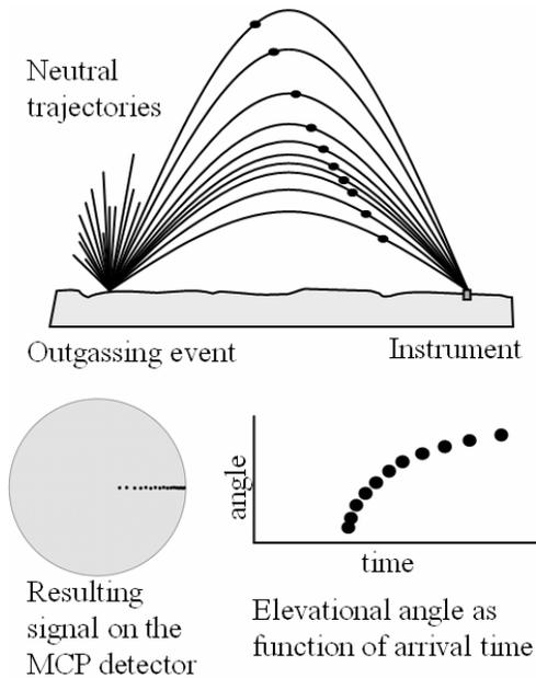
**Figure 2.** Detection of signal from outgassing event.
