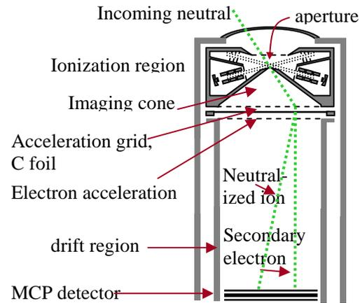
**Figure 1.** Diagram of the LTMS instrument.
