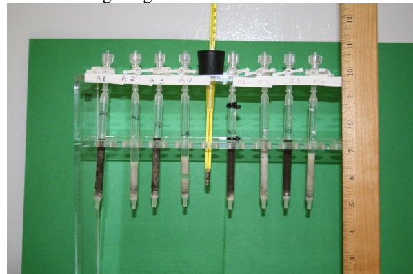
Figure 1. Photograph of columns at the end of the experiment. Bleached columns A2 and O2 were reacted with 0.1N HCl, and A4 and O4 with 0.1N H 2 SO 4 . Unbleached columns A1 and O1 were leached with 0.001 N HCl and A3 and O3 were leached with 0.001 N H 2 SO 4 (A stands for anoxic and O for oxic).
