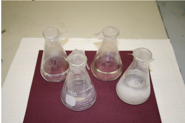
Figure 2. Photograph of precipitates in output solutions from oxic columns (see Figure 1). A similar trend was observed in the anoxic columns.
