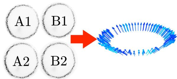
**Figure 1: 3-D PIV Data Set.** Two stereo image pairs of the ejecta curtain “slices.” These images are cross correlated to determine the horizontal and vertical displacements of the particles and, when coupled with the time between successive image pairs, yield the velocity of the ejecta at that moment in time. Images (inverted) are of an impact of a 6.35mm Al projectile traveling at 4.7 km/s at  $90^\circ$  into #20-30 sand.
