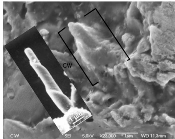
Figure 1: GW tip emerging from fresh fracture surface in an Allende CAI, in an SEM image co-located with a Raman measurement. Inset: Image of synthetic GW showing spindle shape. Scale is different from background image, but note similarities in morphology and size with Allende GW example. Inset adapted from [9].
