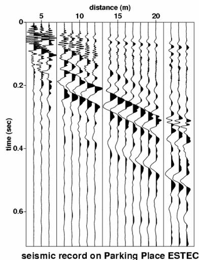
Fig. 4: Test performed with 21 geophones (1-axis) with a hammer trigger in outdoor conditions at ESTEC ExoGeoLab. One can distinguish the air sound wave envelope with a slope consistent with 340 m/s, a refracted wave and a shear wave.
