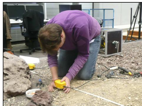
Fig. 3: Tests performed by first author to study the geophone sensitivity according to mechanical coupling to the surface
