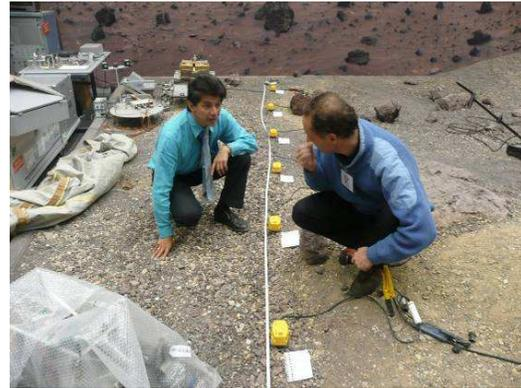
Fig. 1: System of 8 geophones (with 3 axis) deployed and tested inside ESTEC planetary robotic testbed.
