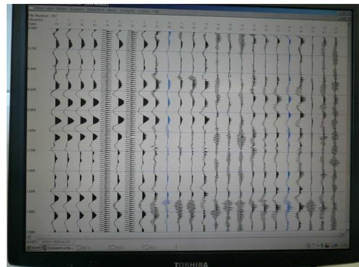
Fig. 2: Quick Look of seismic signal (signal from 8 geophones: vertical, horizontal x, horizontal y)
