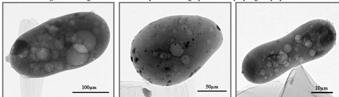
**Fig.3** X-ray ultramicrographs of opaque glassy particles with ellipsoid, teardrop and dumb-bell morphologies.
