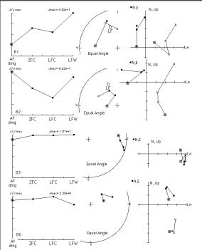
Figure 1: Left panel are magnetic intensity plots in various thermal and field conditions, middle and right panels are equal angle stereonet and Zijdervelt projections of the same data set, respectively. AF dmg – demagnetized NRM starting point, ZFC – zero field cooling to LNT, LFC – application of laboratory field, Jmax in 10<sup>-4</sup>(A m<sup>2</sup>kg<sup>-1</sup>)..
