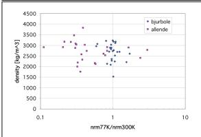
Figure 2: Plot of chondrule densities as a function of their magnetic stability. Magnetic stability is expressed as a ratio between the natural remanent magnetization measured at 77K and the same magnetization measured at 300K
