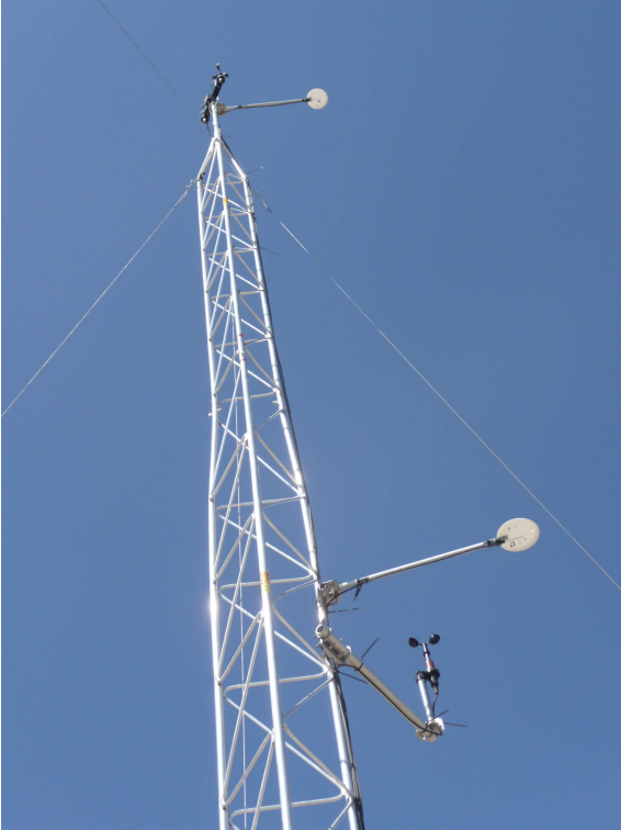
Figure 3: View of the 10m meteorology tower with limited instrument suite. Data from the top anemometer are used for vorticity calculations.
