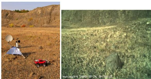
Fig. 3. Hunveyor-4 and Husar-5 rover at the quarry of Hajagos Mountain. Husar rover measures the natural radioactivity of the rocks (left). In the quarry of Hajagos Hunveyor-4 observes the talus of the inner strip pit by camera imaging (right).
