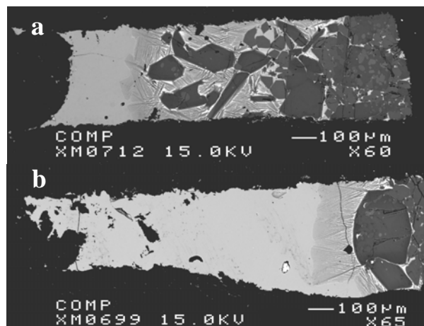
Figure 1. BSE images of Opx-melt partitioning experiments, producing Opx, olivine and melt (1.1 GPa and 1430 °C), a) was doped with Li and b) was not.
