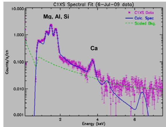
Fig.3. Data obtained by C1XS during a solar flare showing well-defined peaks from Mg, Al, Si and Ca.
